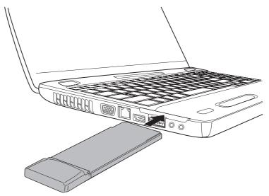
Figure 8-1 Inserting the PC Card
